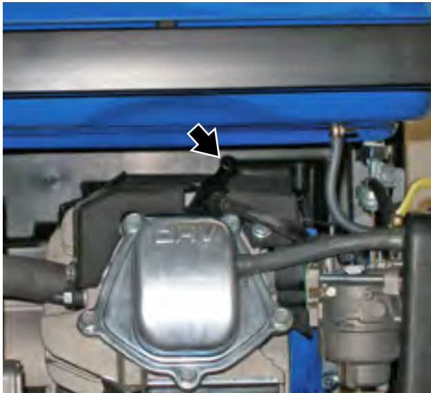
Figure 36 – Removal of Spark Plug Boot
