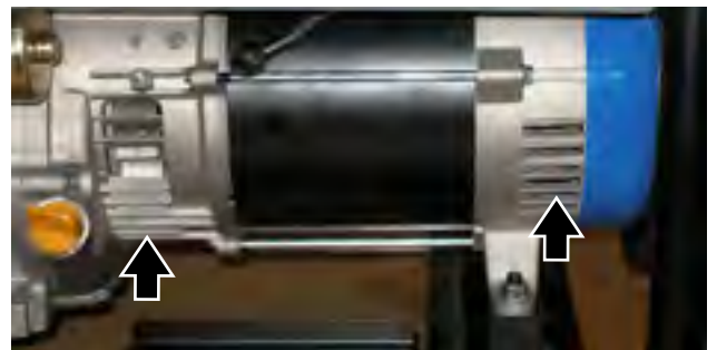
Figure 45 – Alternator Cooling Air Inlet and Outlet Port
